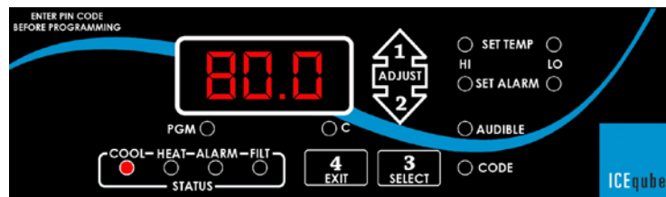
FIGURE 4: REMOTE DISPLAY FOR AIR CONDITIONER.
