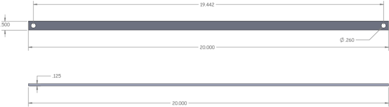
FIGURE 20: 1/2" GROUND STRAP FOR THE LTE SERIES RACK RAILS.
