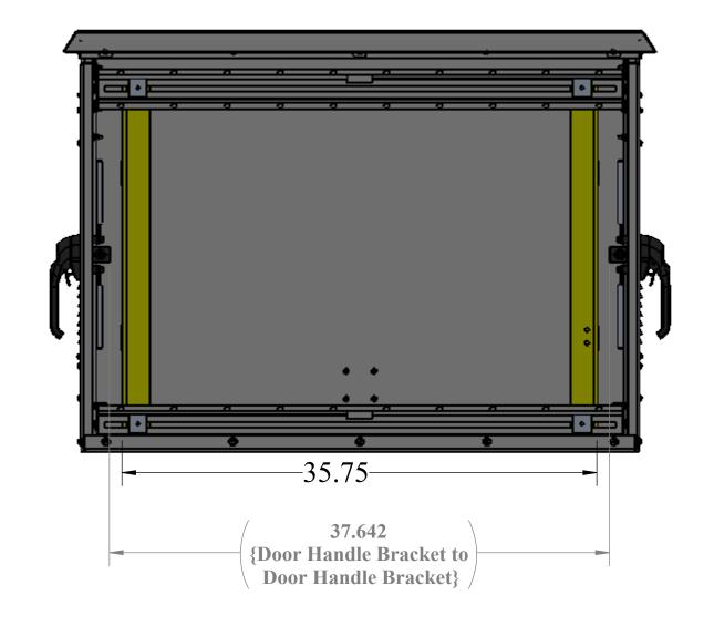
UNLESS OTHERWISE SPECIFIED: DDB Unlimited Inc. DIMENSIONS ARE IN INCHES DX Closed ANGULAR: ±1°
