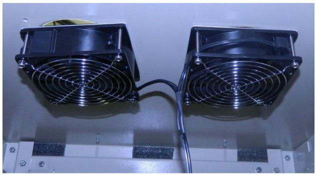
Place the fan screen over the fan and insert screws through the holes and begin tightneing hardware into roof of the enclosure
