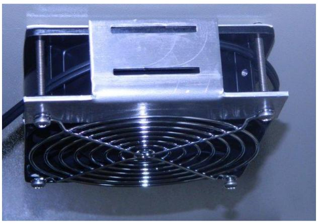
Place Thermostat Bracket onto fan as pictured.
