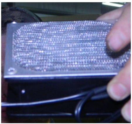
Place the Fan mesh screen on top of the fan, in between the fan and the roof of the enclosure
