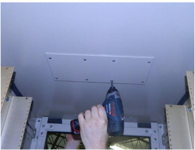
Begin by removing the cover plate in the top of the enclosure as shown above.
