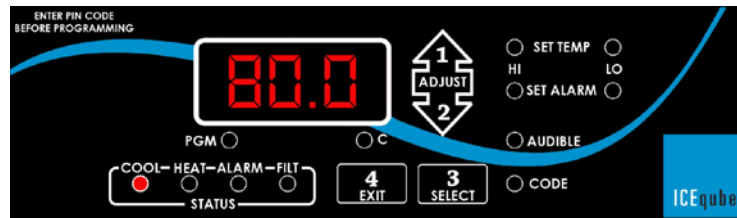
FIGURE 4: REMOTE DISPLAY FOR AIR CONDITIONER.
