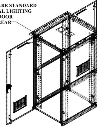
FRONT AND REAR RAILS STANDARD ON DD
