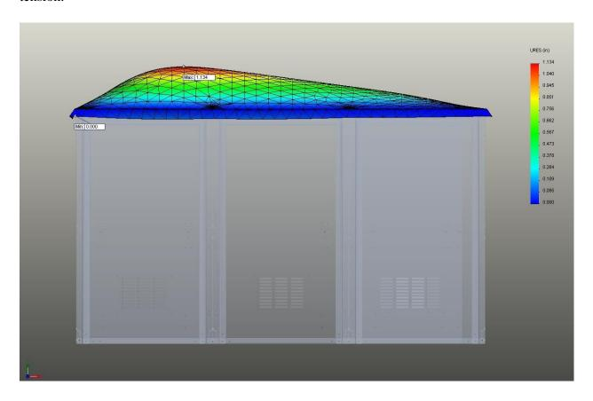
Figure 5: Alumashield Panel Deflection on 3OD (Image from 150MPH Study)
