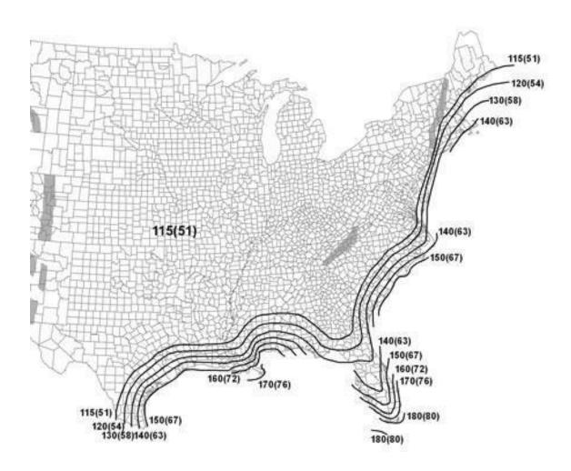
Figure 1: Updated IBC Basic Wind Speeds (ASCE 7-10)
