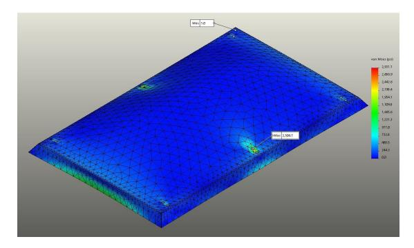
Figure 9: Max von Mises on OD Enclosure in 200MPH Winds
