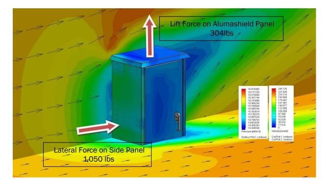
Figure 6: Lateral Pressure on OD Enclosure in 200MPH Winds
