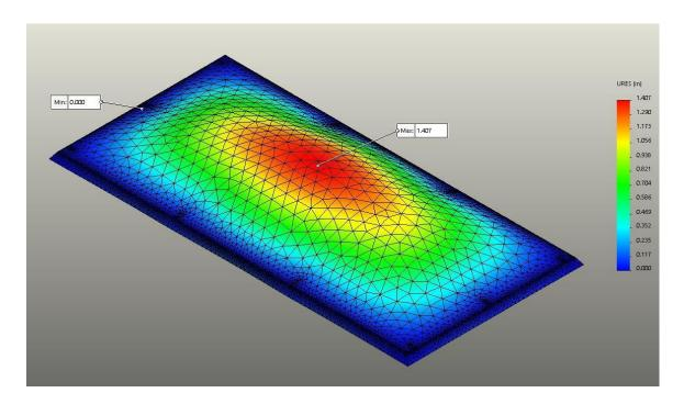
Figure 12: Max Deflection on 3OD Enclosure in 200MPH Winds
