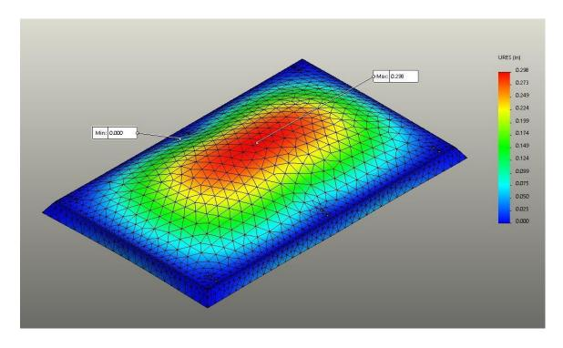
Figure 7: Max Deflection on OD Enclosure in 200MPH Winds
