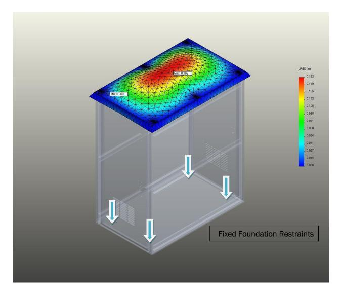
Figure 4: OD Enclosure Fixed Restraints for FEA (Image from 150MPH Study)
