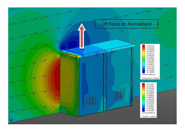
Figure 3: 20D Surface Pressures in 200MPH Winds
