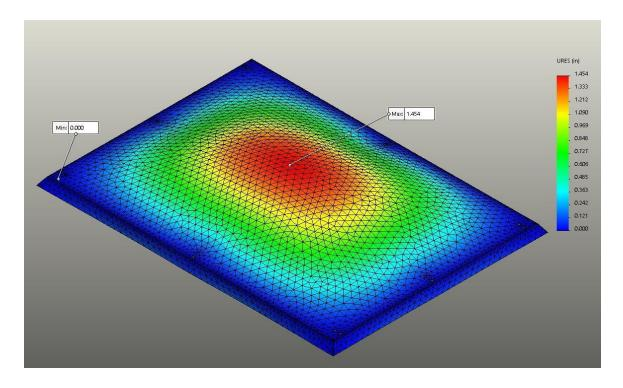
Figure 11: Max Deflection on 2OD Enclosure in 200MPH Winds
