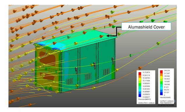
Figure 2: 30D Enclosure in 200MPH Winds
