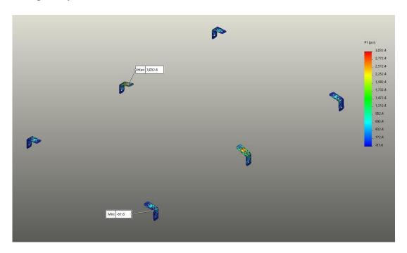
Figure 8: Max P1 on OD Enclosure in 200MPH Winds
